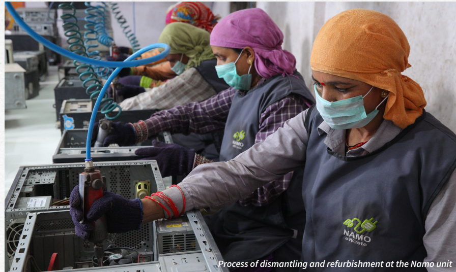
Process of dismantling and refurbishment at the Namo unit
